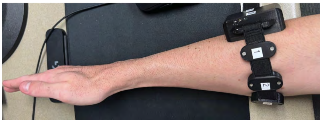
Figure A.3.2. Example of the placement of the EMG cuff on the forearm
