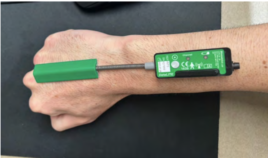
Figure 3.3 Example of goniometer placement on the dorsal aspect of the distal forearm and hand
