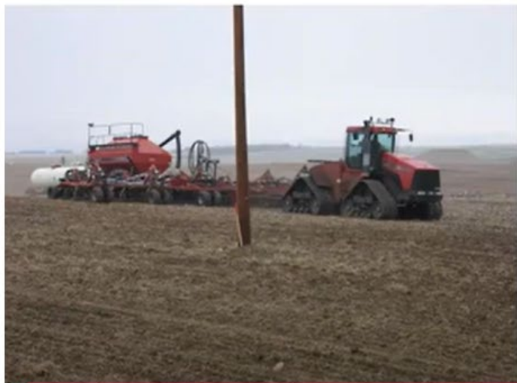
A modern steerable all-tracked power unit planting wheat (Case STX Steiger tractor with Case IH seed drill combination) in western North Dakota, USA. https://commons.wikimedia.org/wiki/File:Wheat_Planting_04_May_2007.jpg
