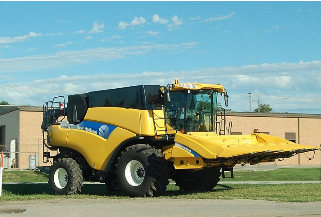
New Holland CR9060 combine harvester with a corn picker header, Beatrice, Nebraska, USA, https://commons.wikimedia.org/wiki/File:New_Holland_CR9060,_Beatrice,_NE.jpg
