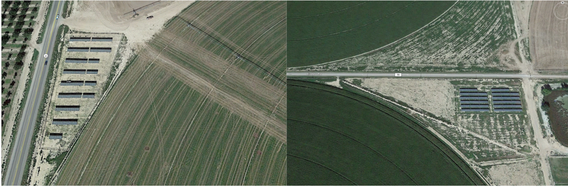
Figure 1 | Center-pivot agrivoltaic systems occupy the corners of crop/pasture fields for solar energy generation but also produce the techno-ecological synergistic outcomes of air pollution reduction, land sparing, food system resilience, and others in Dexter, New Mexico (photo: © 2018 Google; Google Earth).
