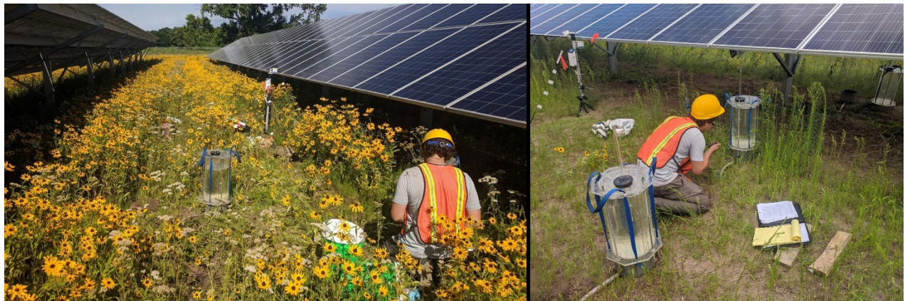
Figure 8. Scientist checks stormwater and soil moisture sensors on an InSPIRE project site.
