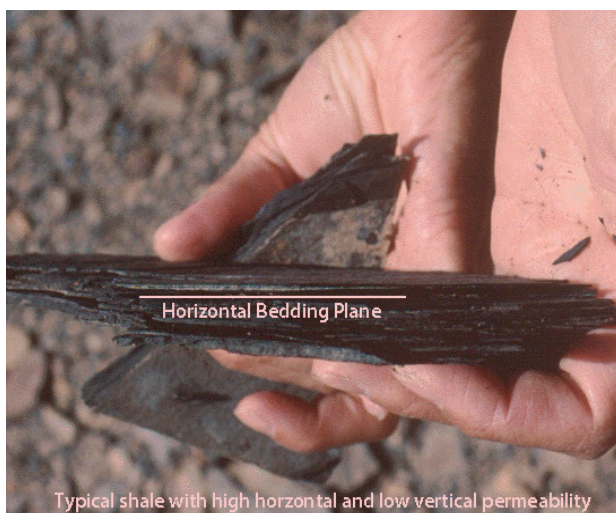
Figure 4: Shale with horizontal bedding planes and low vertical permeability: Source GWPC
