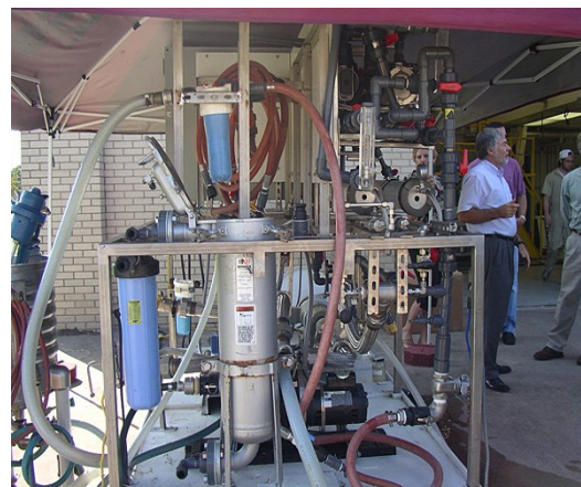
Figure 24: Portable produced water treatment system: Source Texas A&M University and John Veil, Veil Environmental
