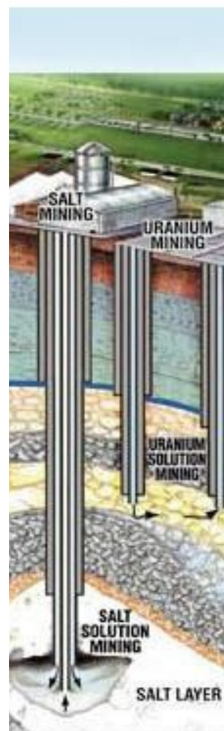
Figure 14: Geologic cross section showing Class III injection wells: Source, USEPA
