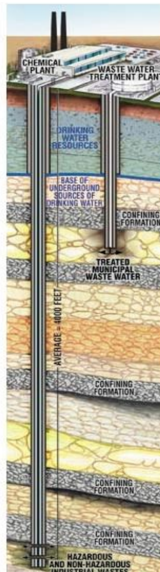
Figure 8: Geologic cross section showing Class I wells: Source USEPA
