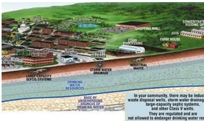
Figure 15: Geologic Cross section showing Class V injection wells: Source USEPA
