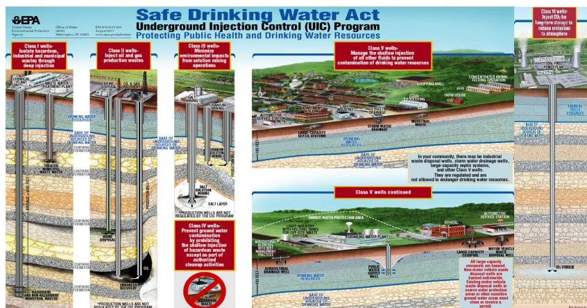
Figure 5: UIC Program Well Classes: Source USEPA
