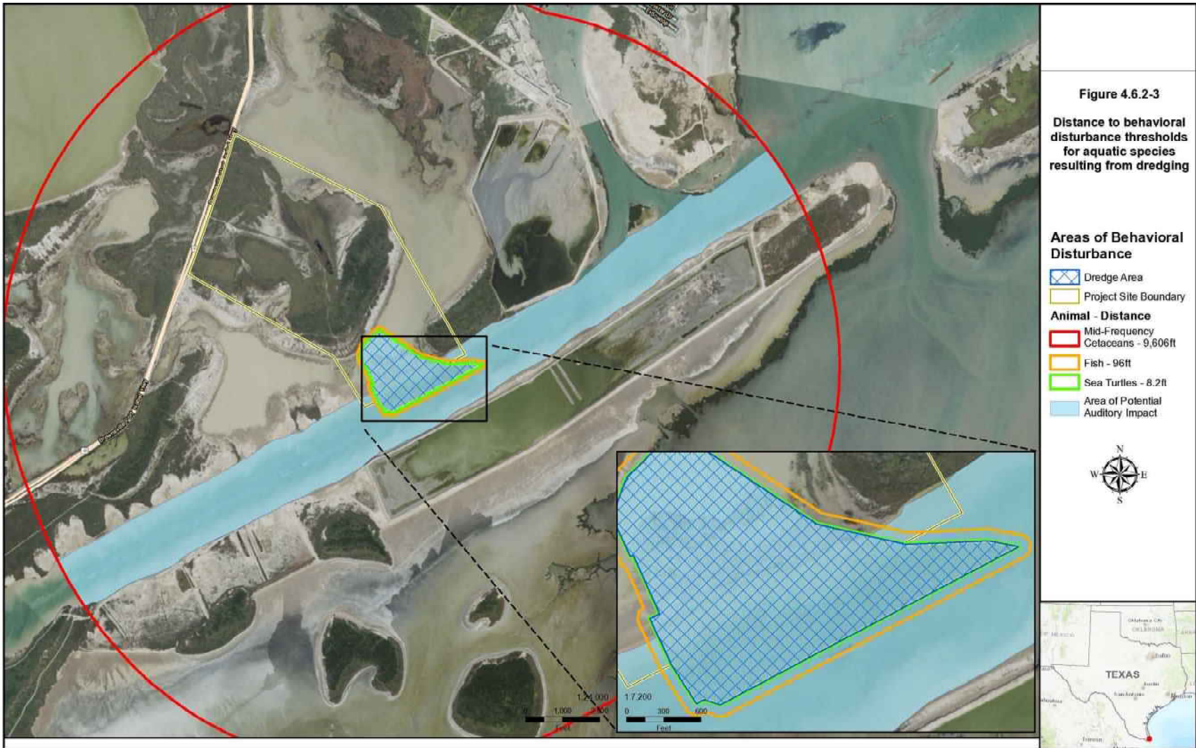
FIGURE 4.6.2-3 Distance to behavioral disturbance thresholds for aquatic species resulting from dredging.
