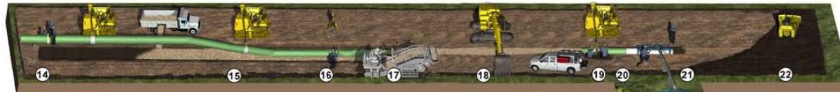
14. Inspect and Repair Coating 15. Lowering-in 16. As-built Survey 17. Pipeline Padding (as needed) 18. Backfill and Preliminary Clean-up 19. Tie-ins 20. Pressure Testing, Final Tie-in 21. Calliper Run and Calibration Digs 22. Clean-up, Restoration, & Seeding/Mulching
