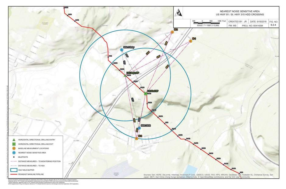
Figure 4.10.2-2 US Hwy 81 / St. Hwy 315 HDD Site: NSAs and Ambient Sound Level Measurement Locations
