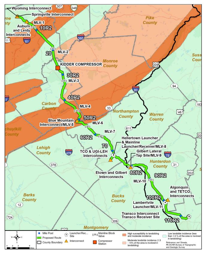
Figure 4.1.5-1 Landslide Potential Near the PennEast Pipeline Route
