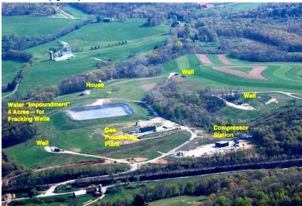
Figure 25: Aerial view of a shale gas well site in the Marcellus Shale Gas Field – house and nearby gas operations.
