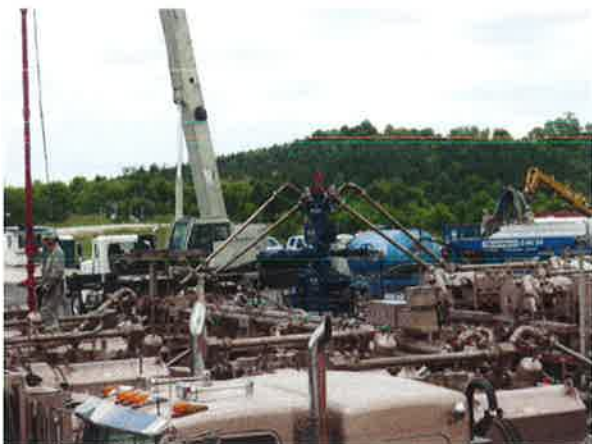
Figure 12. A HF well (blue, center) connected to piping containing fracture stimulation fluid pressurized from pump trucks. Mouser photo.
