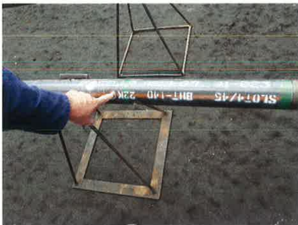
Figure 1. Example perforated casing containing spiraled charge detonation points for focused fracture stimulation. Mouser photo.
