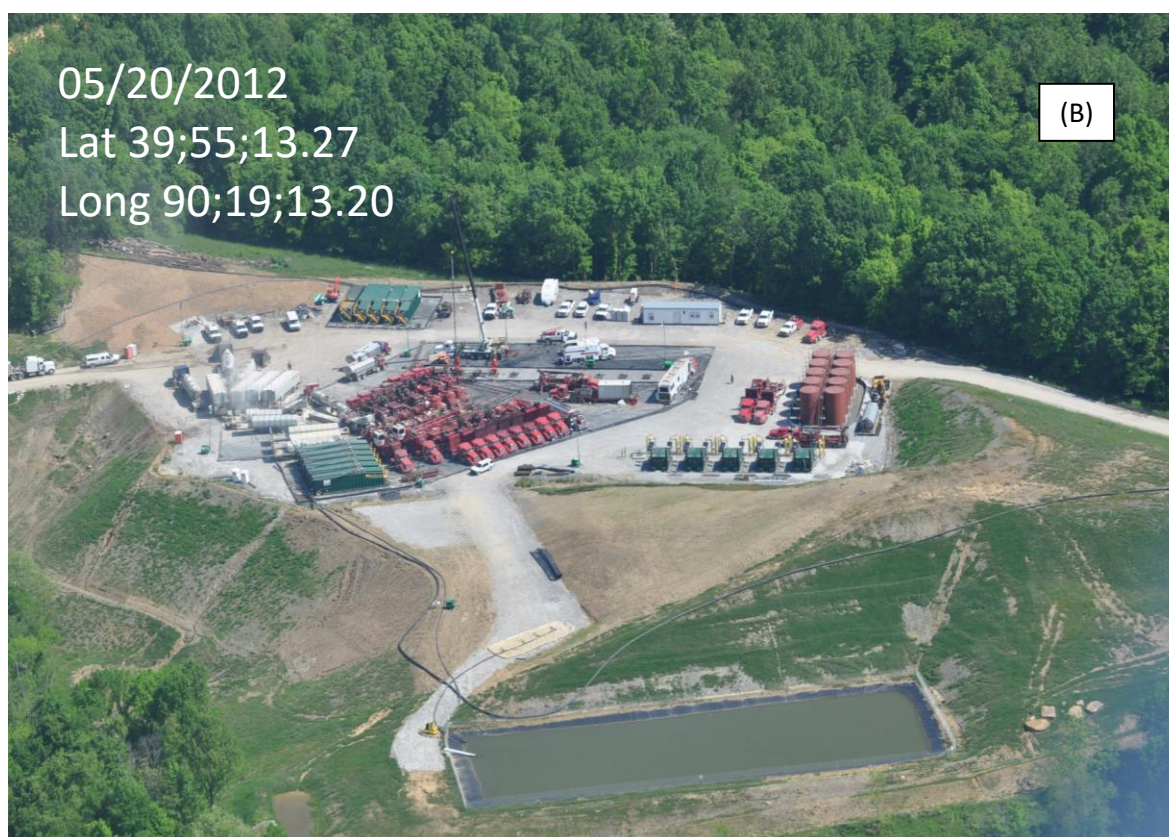
Figure 6. (A) Typical Marcellus shale gas multi-well pad during drilling operation. (a) Drill rig; (b) Unlit but venting flare stack; (c) Air compressors; (d) Main high-pressure air-line; (e) Flow line; (f) Separator unit; (g) Water tanks. (B) Typical Marcellus shale gas multi-well pad during stimulation operation. Note large water impoundment, lower center.
