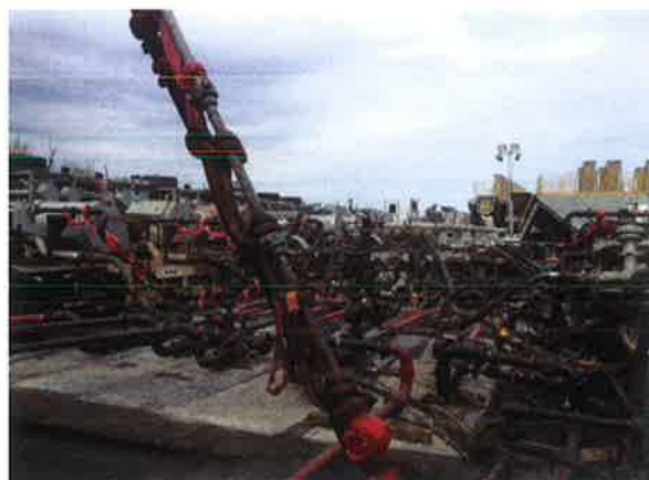
Figure 13. A close-up of fracture stimulation fluid piping connected between blender, pump trucks, and the wellhead. Mouser photo.
