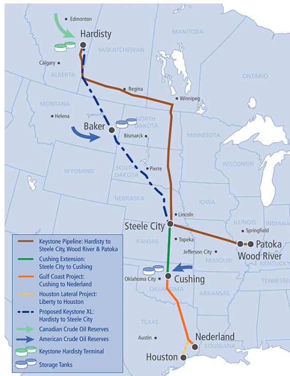
18. TransCanada commenced preparations to build the Keystone I Pipeline and Cushing Extension in 2005. The Keystone I Pipeline extends from an oil supply hub near Hardisty, Alberta to terminals in Illinois and transports crude oil produced from areas often referred to as the “oil sands.”
