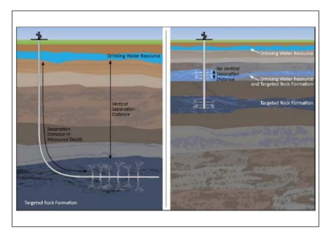
AR BI 13430 (figure 2, from EPA's Hydraulic Fracturing Report, depicting examples of hydraulic fracturing with a relatively large separation distance between the shallowest fracture initiation depth in a well to the base of the
