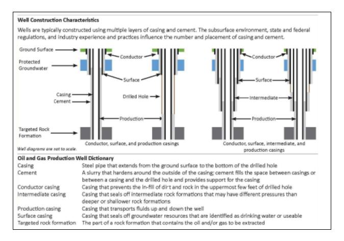
AR BI 13066 (figure from EPA's Hydraulic Fracturing Report, depicting oil and gas wells with surface casing extending below protected groundwater).
