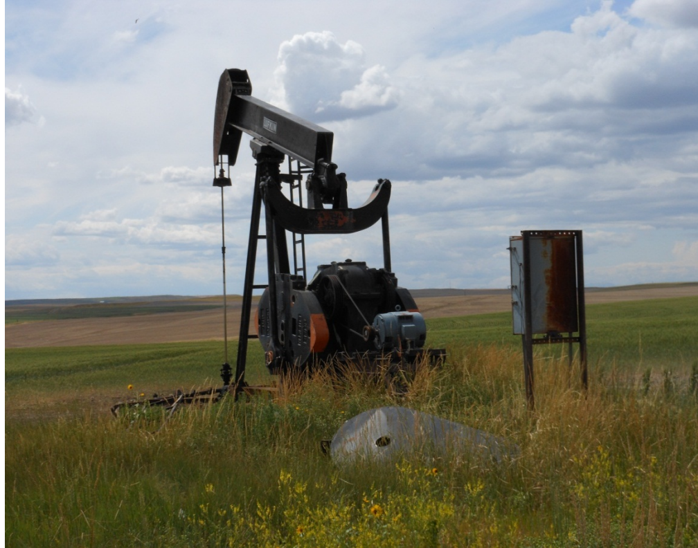
Figure 3. Pumping unit used for producing oil on tribal lands. Photo by OIG.
