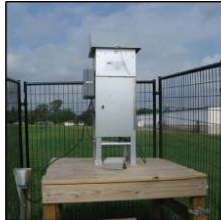
High-volume TSP Sampler
