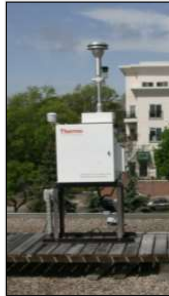
Low-volume PM 2.5 filter monitor
