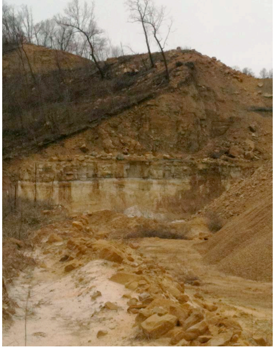
The light area in the exposed hillside of the Pattison Mine in Clayton County shows a deposit of the sand sought for hydraulic fracking operations. David Osterberg photo
